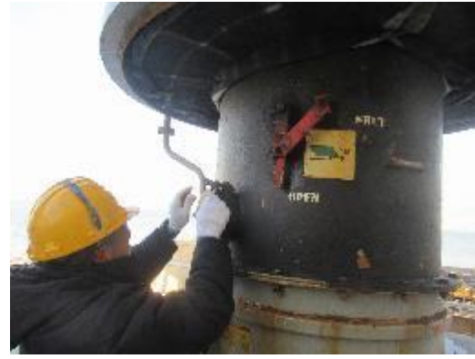
The hand levels were found rusty, advised to maintenance by chipping and scrapping
