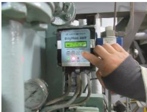
15ppm alarm test, result ok
