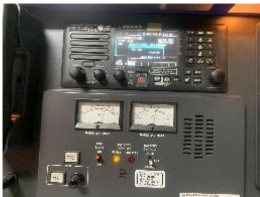
MF/HF DSC test, dropped down to 22V after
