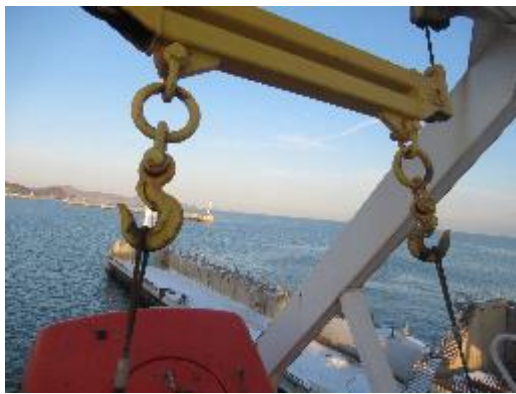
The latch of hook for boat falls were found clogged, advised to fair up and greased up
