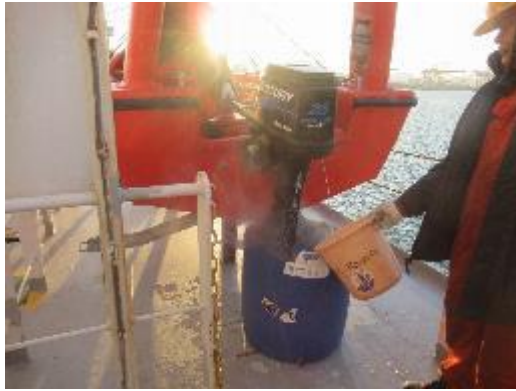
Functional test for rescue boat engine is ok
