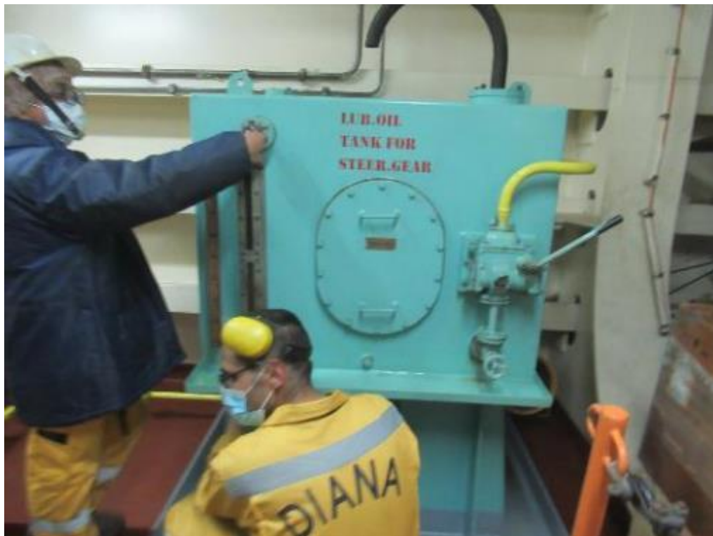
No.18 : the min level of oil gauge for LO steering gear oil tank not marked in place.
