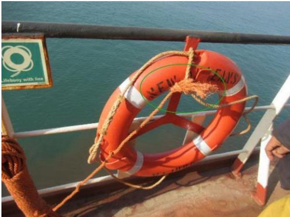
Picture 9: –Lots of wrongly connected between life buoy and life lines were observed.
