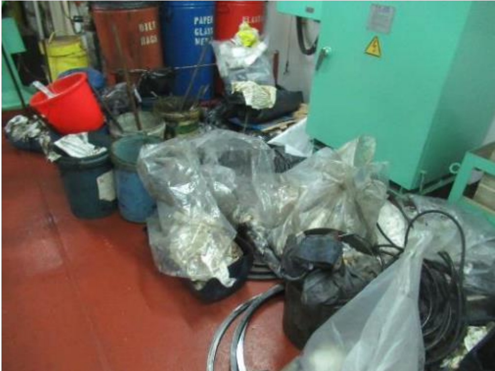
Picture 13: - Lots of oil rags were observed not improperly collected stored in suitable steel drum to prevent possible fire
