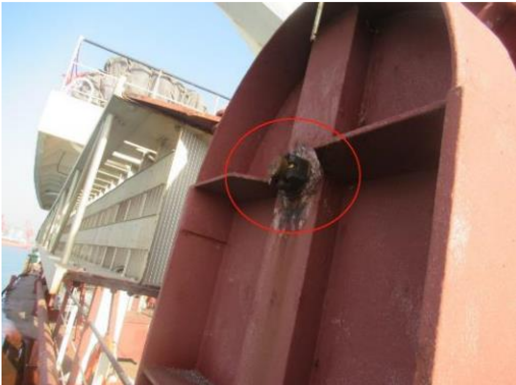
Picture 12: the turntables for accommodation on port side was found rust and obstructed, advised to fair up and grease up for freely operation.
