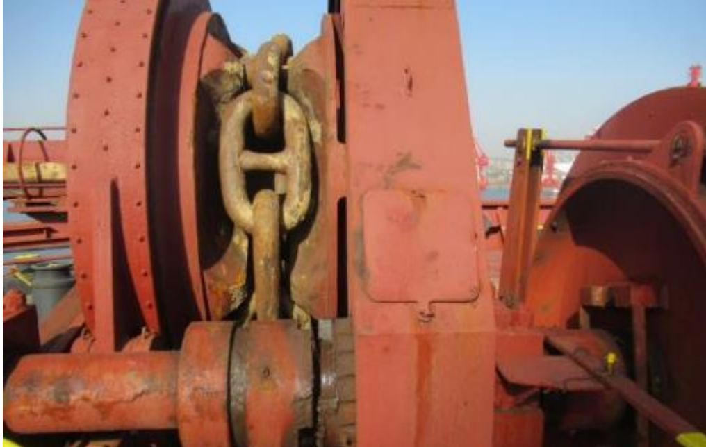
Picture 1: The grease windows for both anchor was found clogged.
