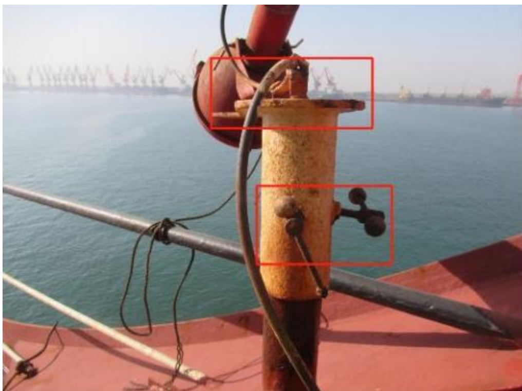
Picture 10: Lots of light pedestals for lighting system was found obstructed and clogged by paint and heavy rust. And tightening bolts also found wear down, advised to thoroughly check and repairing
