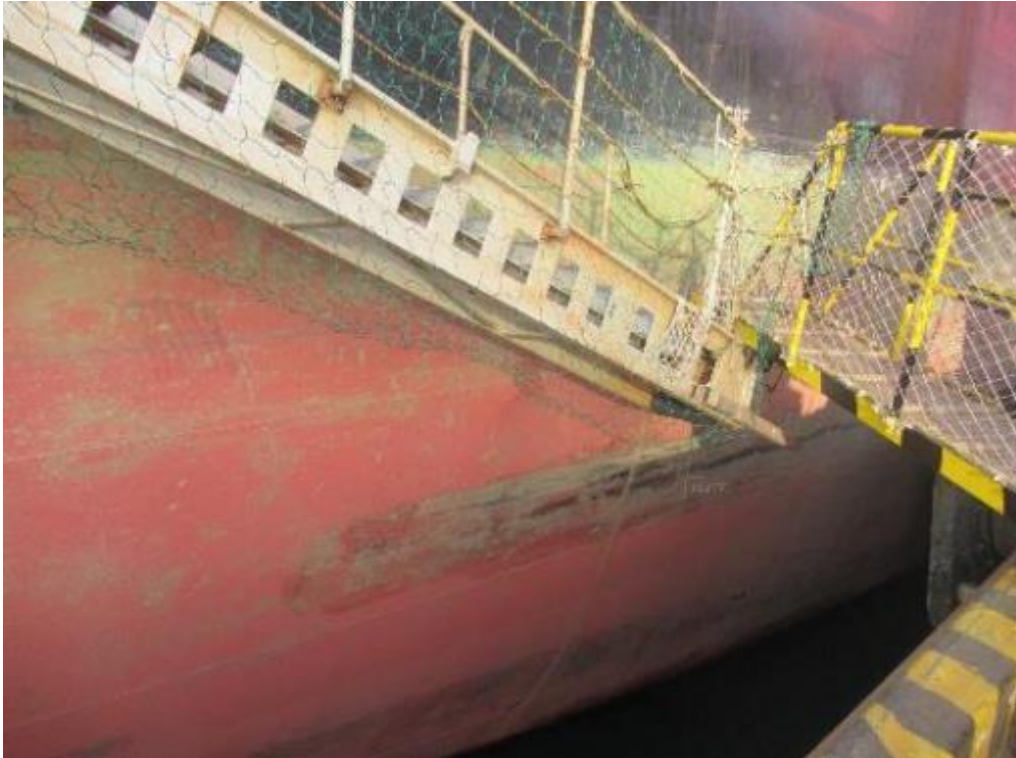
Picture 10 : the brow ladder supplied by shore side not protect with safety nets in compliance with AMSA recommendation
