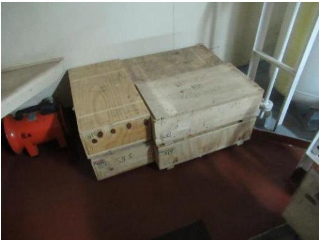
No.16 : Lots of newly supplied spare box in engine room were found not sea fastening for safe purpose.
