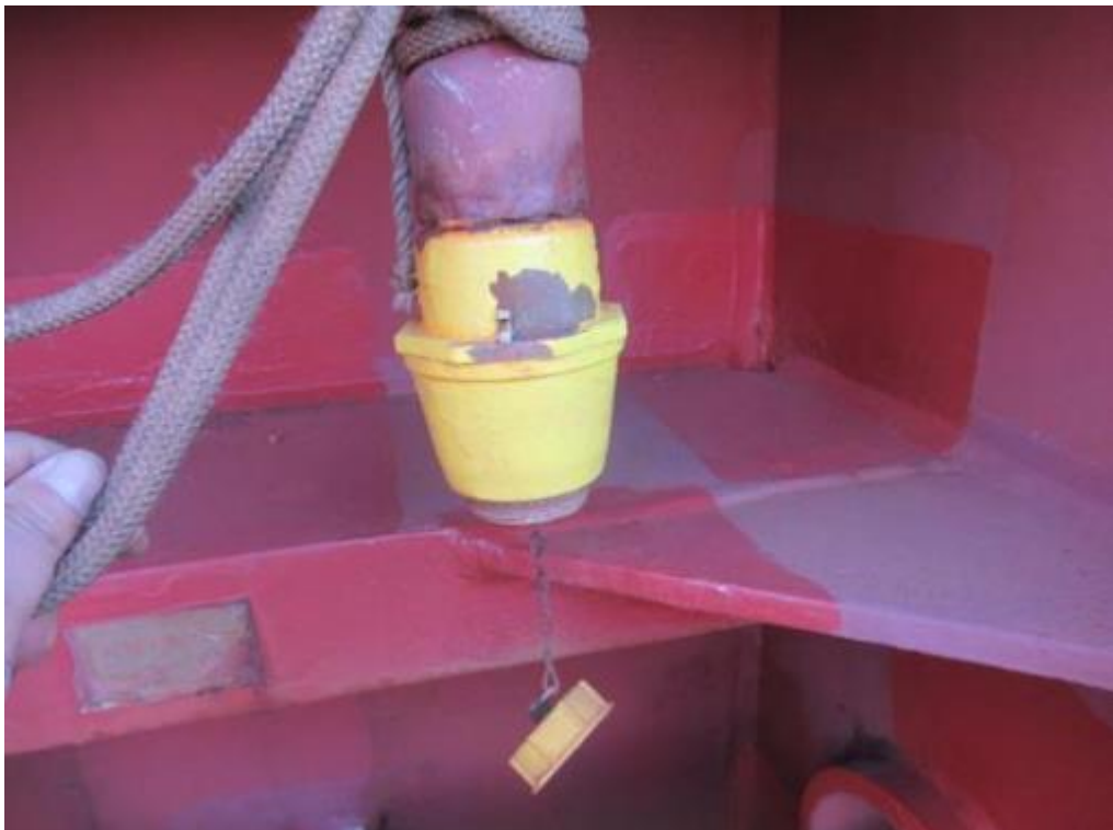
Picture 2: Some of the drainage balll acting as non return valves was found cloggd by foreigh materials.
