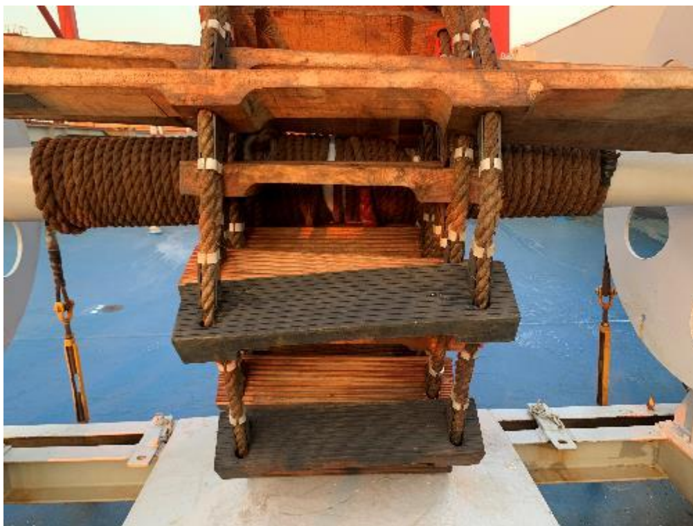
Picture 21: the step space of pilot ladder on gear on the starboard side was found not marked at regular intervals with meters
