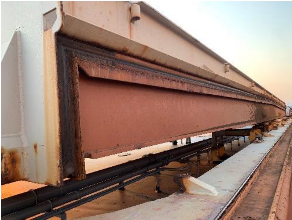
Picture 22: The spot rust on hatch coming area and double sweat channel were observed.
