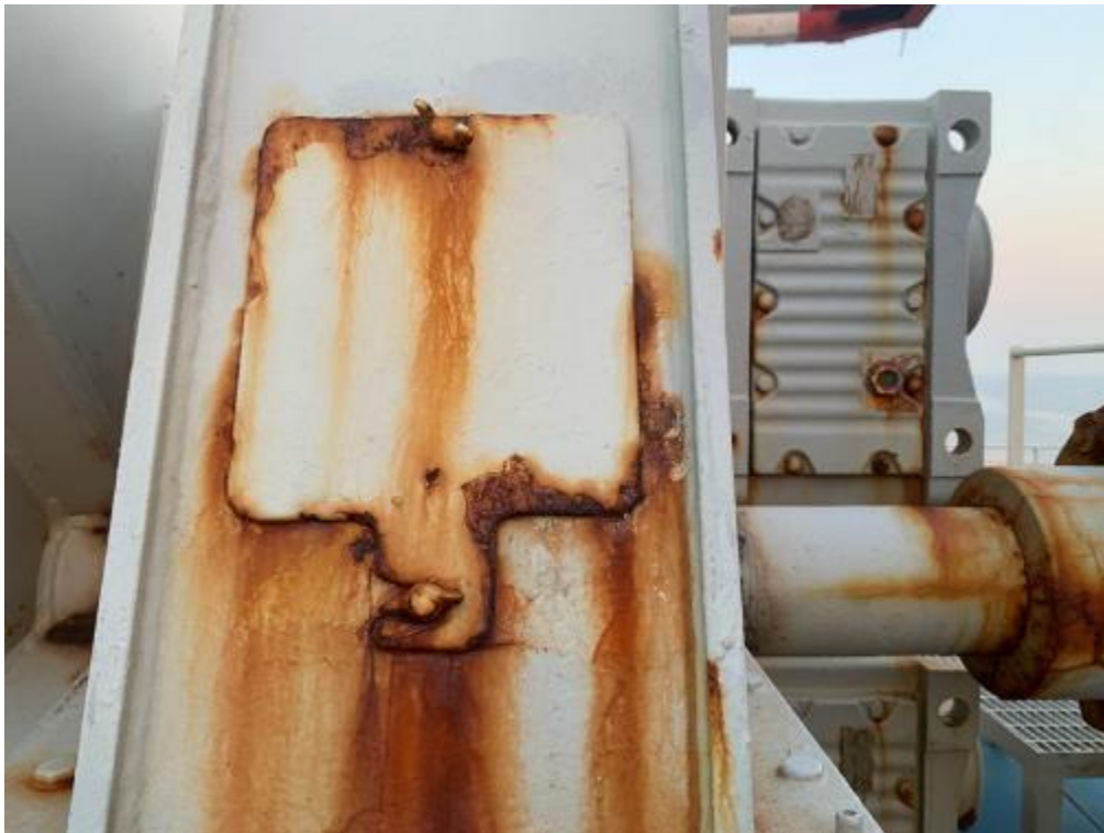
Picture 5: - 1.the mooring winch with grease windows was found heavily rust.
