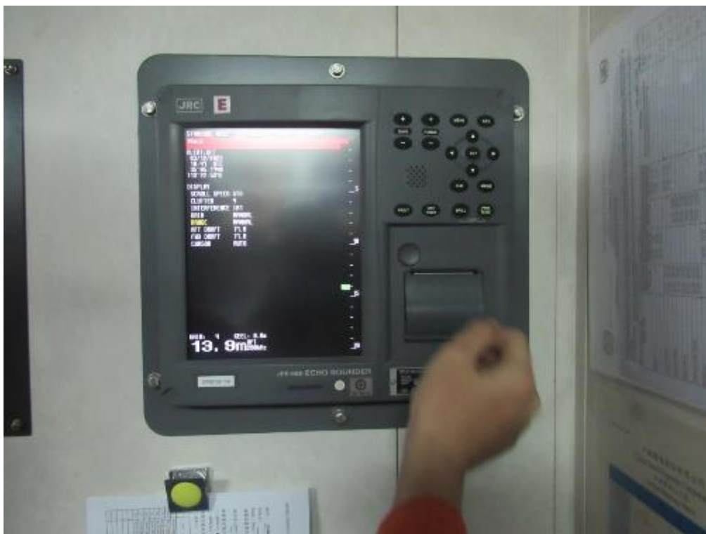
Picture 3 : the UKC setting in echo sounder was found incorrect
