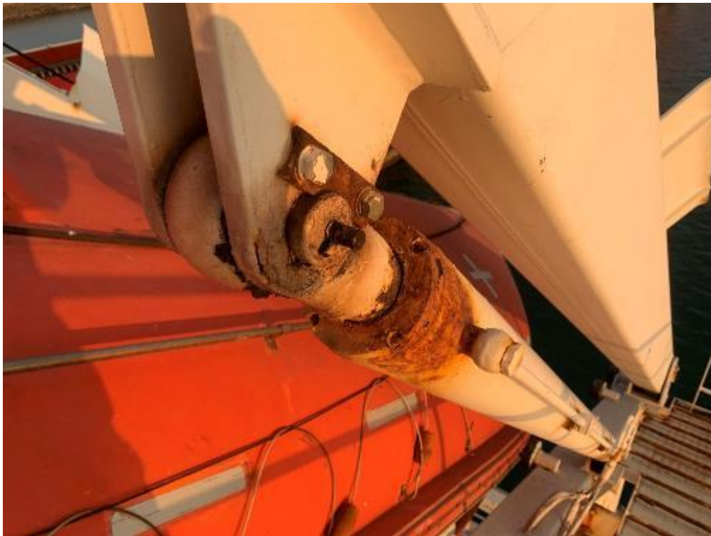
Picture 19-1: Rust on the hydraulic jack and davit for freefall lifeboat was observed, advised to maintenance and greased up as per PMS requirement
