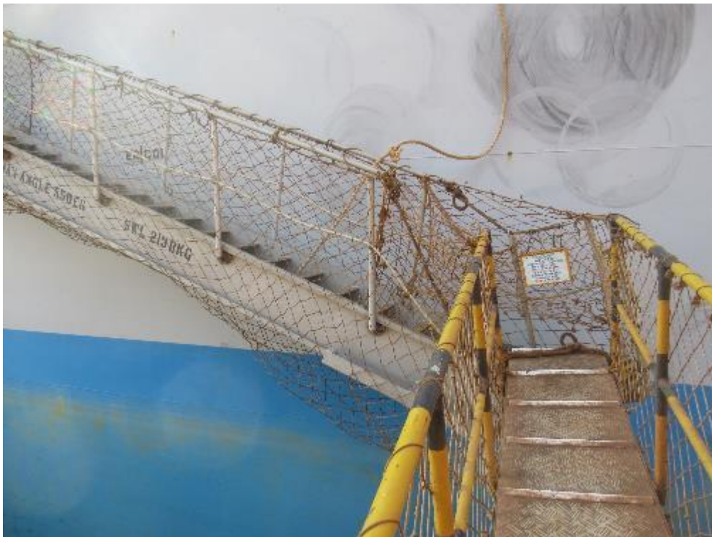
Picture 16: -The shore brow gangway attached to the bottom platform was found not improperly protect with safety nets .
