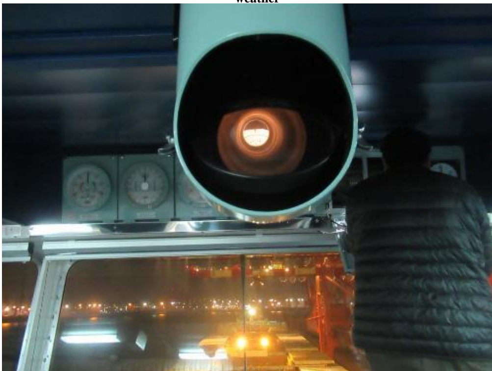
Picture 2: the Magnetic error was found more than abt 16 degree after compare with Gyro Compass
