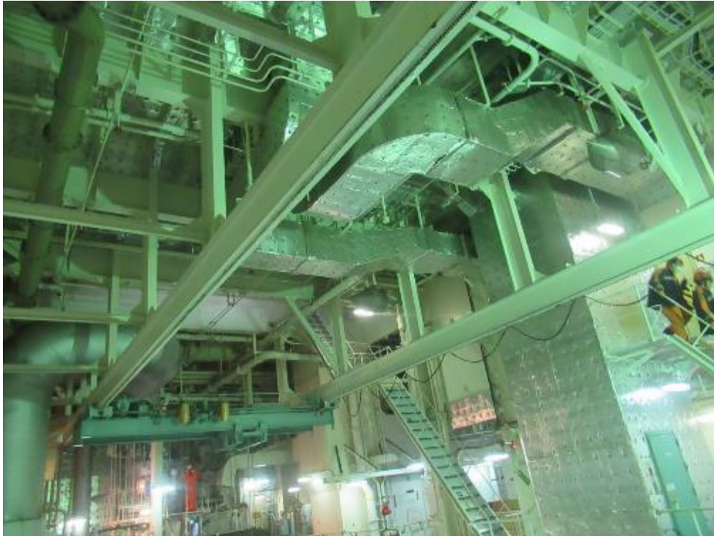
Picture 12: - Engine room over head trolley cranes SWL was marked only on one location
