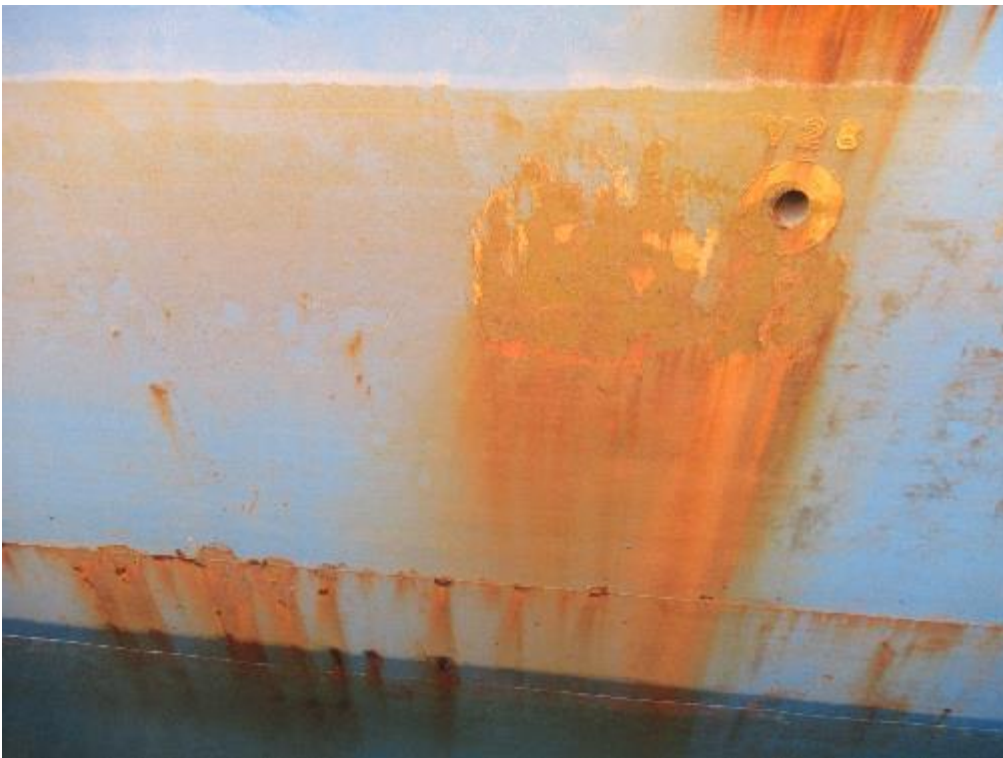
Picture 23: The side hull on the port side was found rust and partly scratched, advised to derust and touch up .
