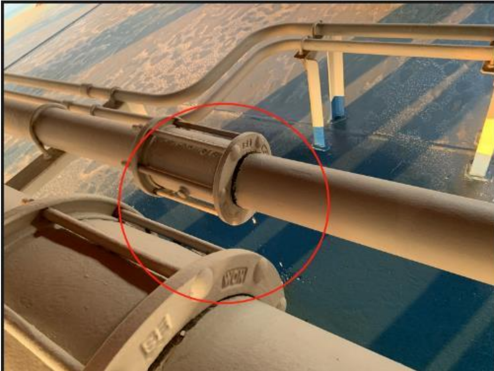
Picture 17: Expansion joint on fire lines on port side in way of about frame No. 60/90/265 were found leakage.
