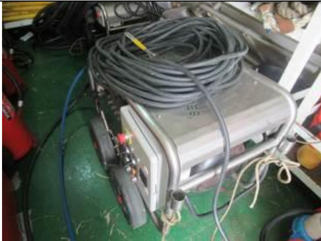
HP Machine (500Bar, testing at 380Bar)
